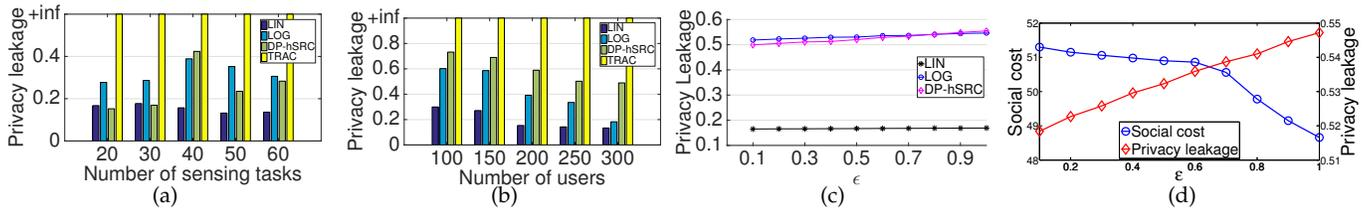
Fig. 6. Evaluation of privacy leakage for BidGuard. (a) Impact of the number of sensing tasks. (b) Impact of the number of users. (c) Impact of  $\epsilon$ . (d) Social cost v.s. privacy leakage.
